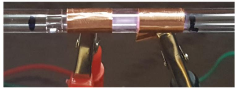
Figure 5 Cold helium plasma between two electrodes inside a quartz tube.
