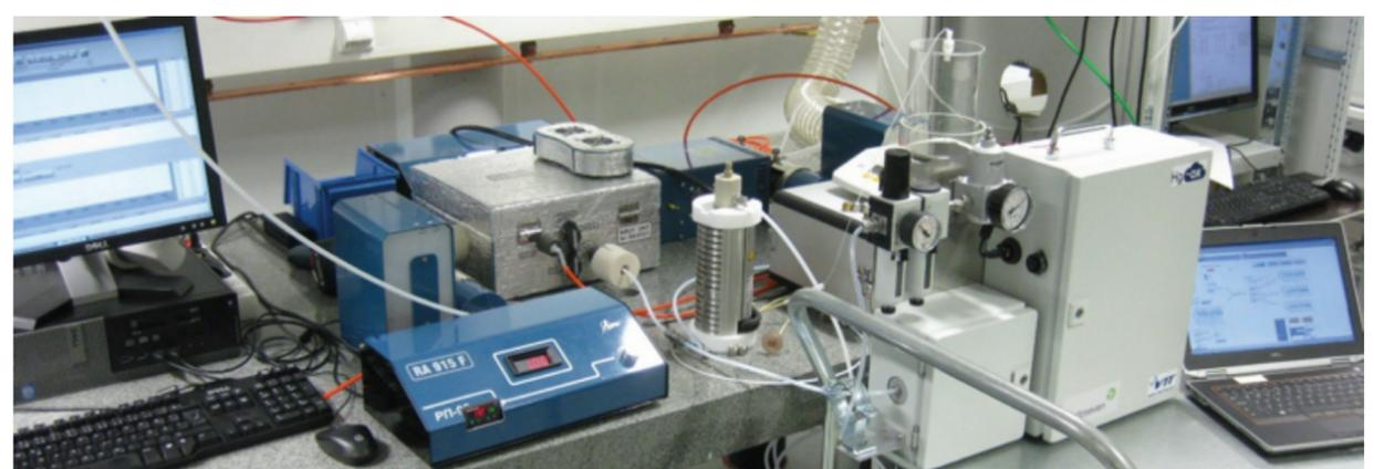
Figure 2 Setup of the two channel analytical system (left) and liquid evaporative  $\text{HgCl}_2$  generators (right).
