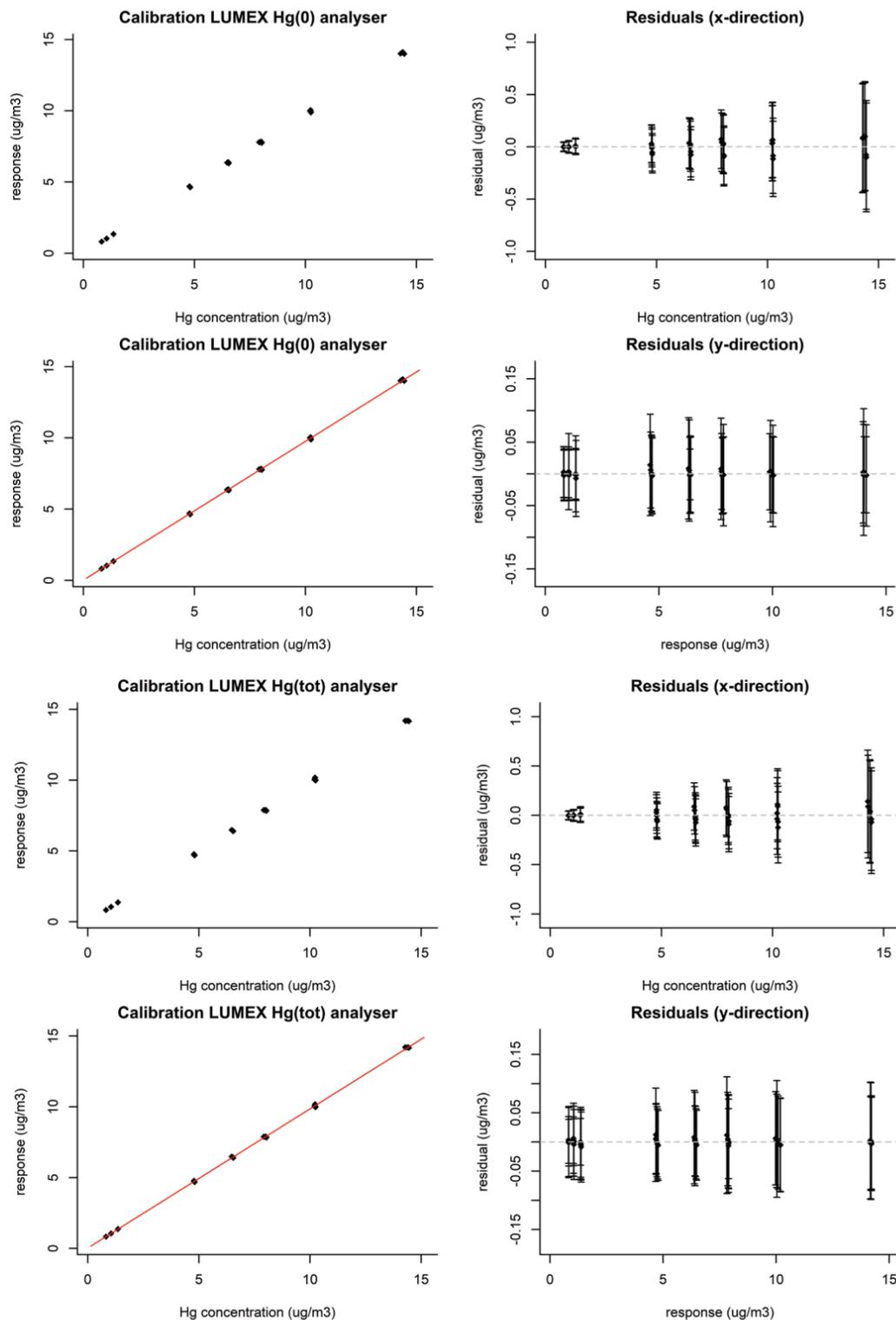
Figure 3 Calibration of both channels of the two channel analytical system, including the residuals calculated according to ISO6143.
