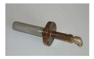
Fig. 3: Amalgamation of mercury on a gold trap
