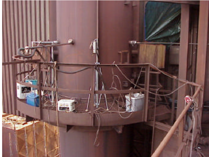
Fig. 1. Sampling equipment at the iron-ore grinding installation.
