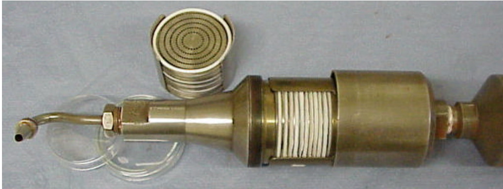
Fig. 3. The Andersen cascade impactor, opened after the sampling of iron-ore dust.
