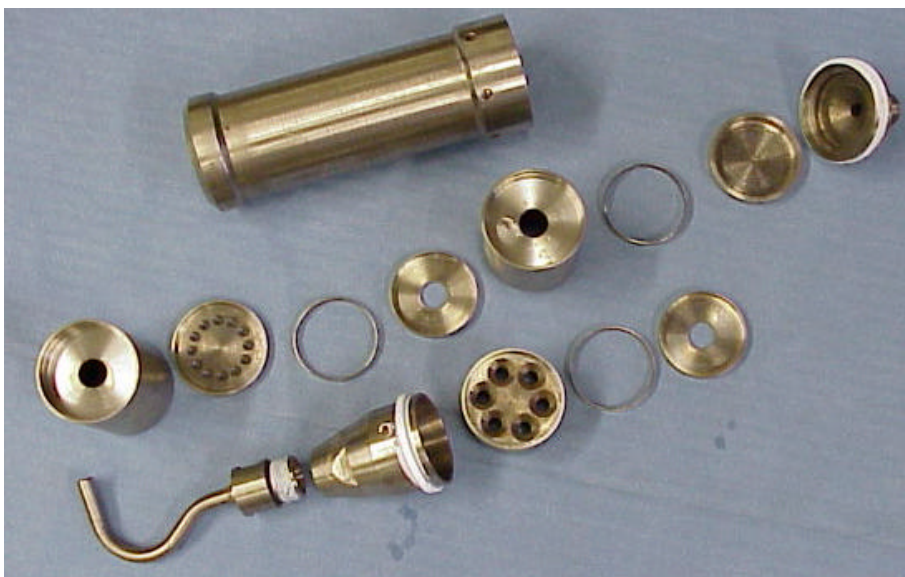
Fig. 4. The Johnas probe, opened after sampling of iron-ore dust.
