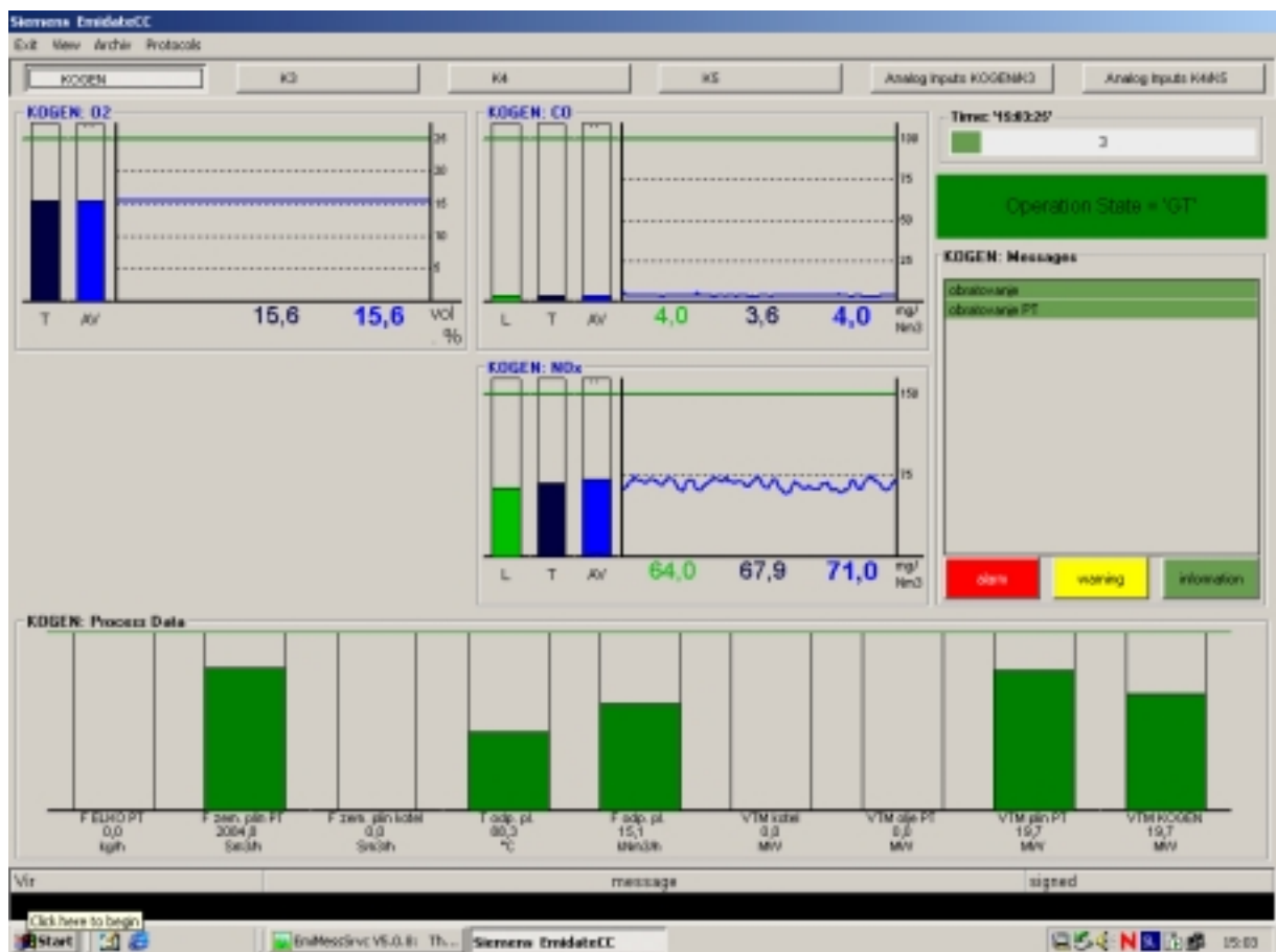
Figure 3. Display of EMIDATE AES (Automated Evaluation System) at Energetika Ljubljana SLO.
