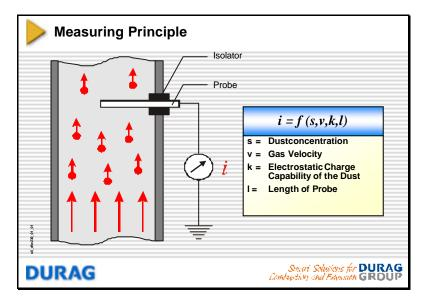
However, if the gas velocity is measured in parallel and the triboelectric reading automatically corrected for velocity changes this methodology can also be used for quantitative dust concentration measurement and can be calibrated using the standard method.
