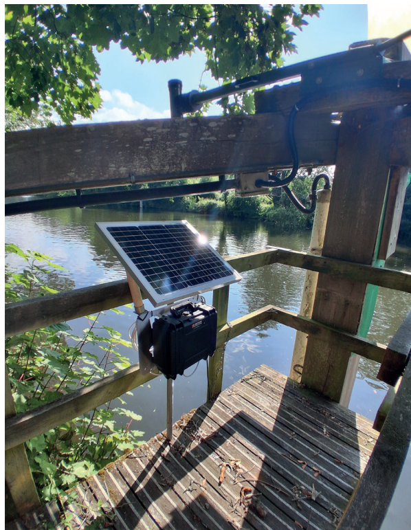
Portable ESNET Water Quality Monitor, River Medway
