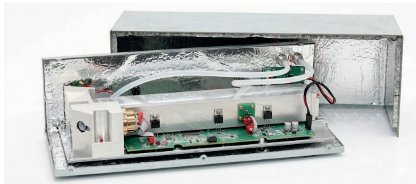
Figure 5: SPECTRO.sens optical bench with signal processing electronics integrated into the thermal housing
