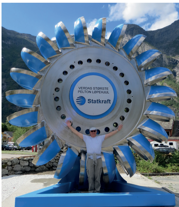
Claimed to be the world's largest electricity generating Pelton Wheel, this example is installed at the Eiriksdal Hydropower Plant in Norway and generates up to 30MW of power.
