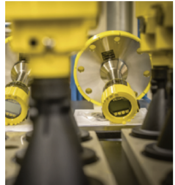
The customer simply orders a VEGAPULS 6X. The exact appearance and configuration of the finished measuring instrument is determined by the application. The radar sensor is custom-assembled at VEGA on the basis of the specified parameters and process conditions.
