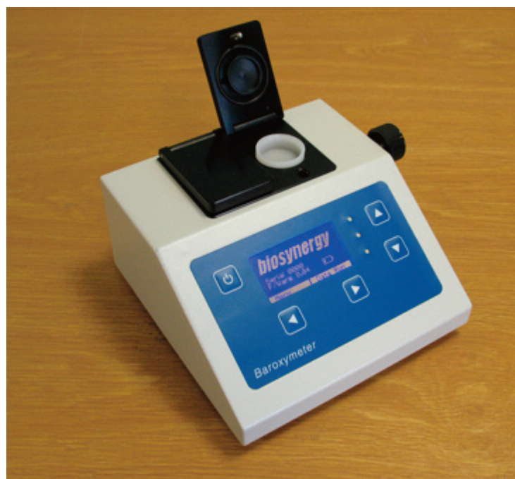
Figure 1. The Baroxymeter: a portable respirometer for the detection of toxicity in wastewater.
