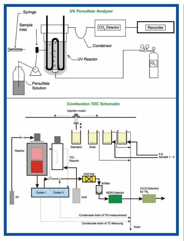
Over the years there have been advancements made in UV persulfate methods and the analyzers utilizing this methodology. One area that has seen improvement is the advent of more efficient high-energy UV sources. Modern lamps have the ability to produce strong UV emissions at 185 nm and 254 nm, which stimulate the production of hydroxyl (OH.) free radicals in the solution being analyzed. It is these free radicals that assist the oxidation of the organic compounds in the sample.
