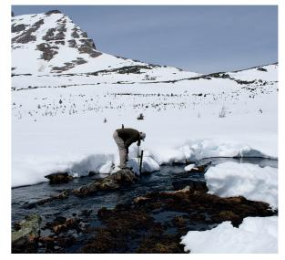
Solinst Levelogger Recording Water Levels in an Alpine Lake Stilling Well
