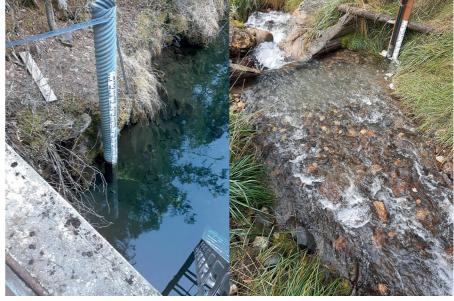
Solinst Leveloggers are Installed in PVC or Steel Pipe in Streams to Record Water Levels
