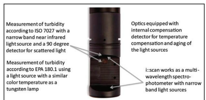
Figure 1: 180° spectral absorption measurement with 90° light scatter measurement combined in a single instrument
