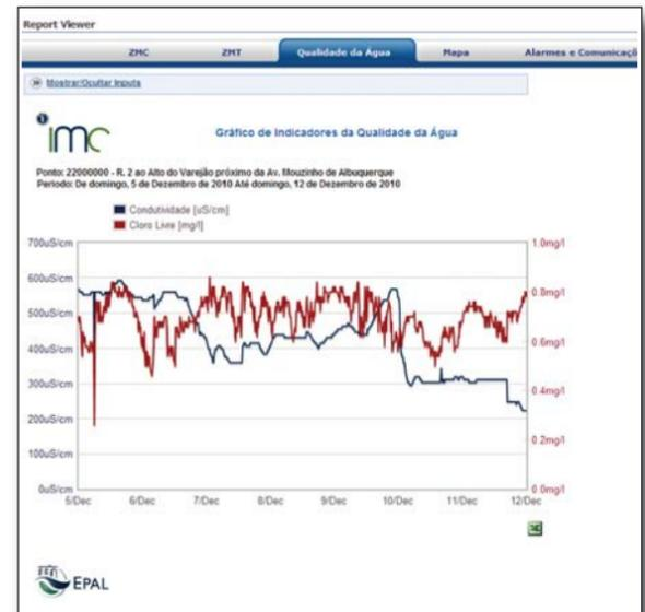
Figure 1: Example display showing Continuous Free Chlorine and Conductivity readings
