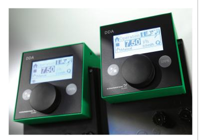
The large LC display, which is clearly visible from some distance, indicates the pump status. If the display is green, the pump is operating and everything is as it should be. In the event of a fault, such as an empty level signal, the display turns yellow (warning). A red background is used for an alarm situation, while white indicates that the pump has stopped.
