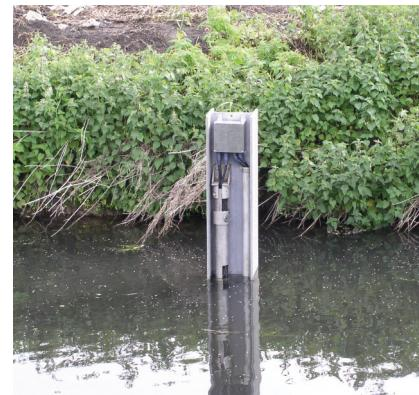
After considering a number of flow measurement options, CEMEX asked Flowline to provide a metering station which would continuously measure the river flows to provide data for use in calibrating a hydraulic model of the Erewash and Attenborough lake system. Another important consideration was that the site was open and accessible to the public and incidents of vandalism had occurred, so any equipment installed had to be as robust as possible, without being too intrusive.
