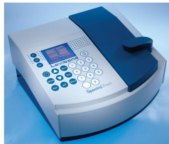
The SpectroDirect is a modern single-beam spectrophotometer with an excellent price/performance ratio that is specifically designed for water testing.
