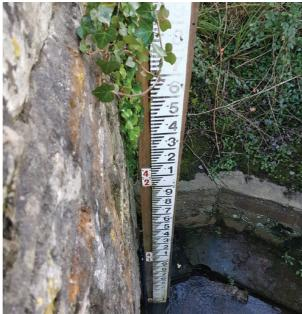
Wardens and residents could then request water level data via SMS from the LeveLine-EWS, obtain the reading and translate to the threat of flooding, all without leaving the house. And critically, to erect flood boards in plenty of time to protect homes. An important by-product was that it reduced the number of times boards were erected unnecessarily.
