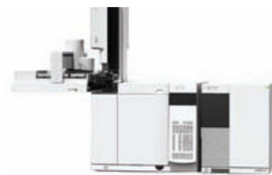
The Agilent 240 Ion Trap MS connected to the Agilent 7890A GC
