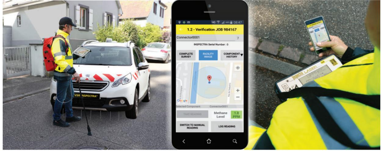
The INSPECTRA LASER technology equips network survey vehicles and portable detectors for the leak inspection of gas distribution networks. New communication technology makes it possible to connect wirelessly detectors, mobile phones, tablets and PC interfacing with a global enterprise management system. Leak data is sent out to concerned parties for immediate analysis and processing.
