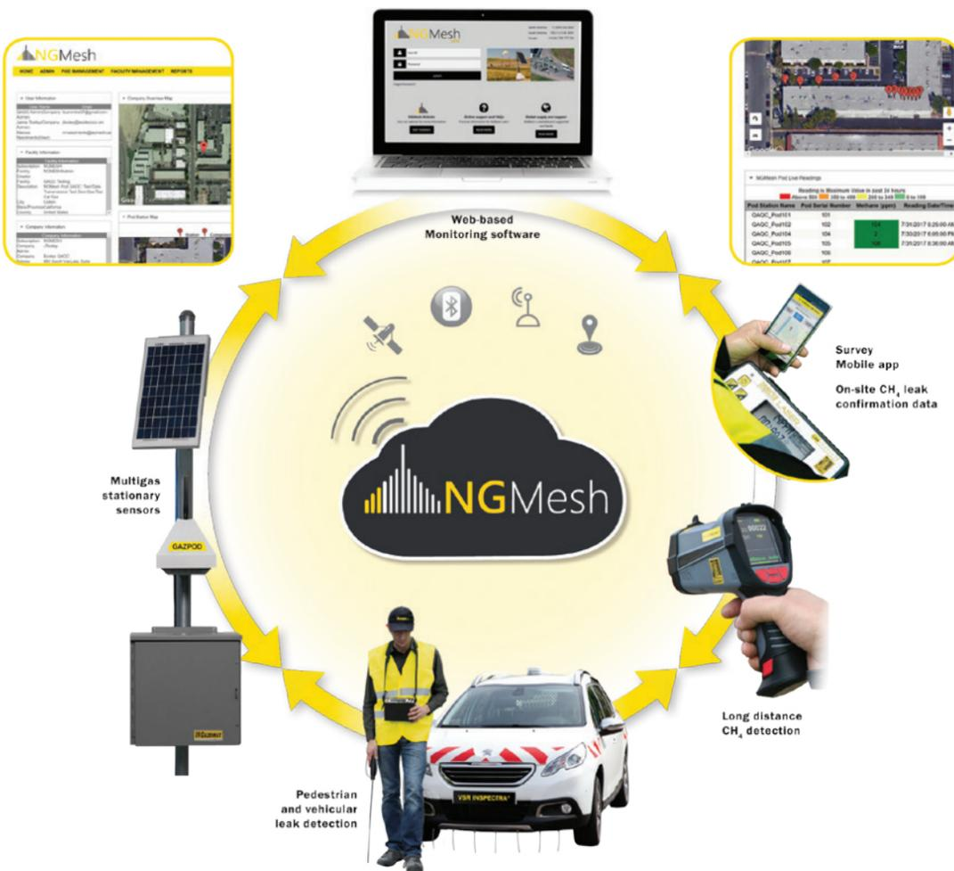
Example of a BIG DATA approach where leak detection instruments and data collecting devices all interface with an enterprise system that can manage hundreds of leak detection systems running simultaneously in different locations with hundreds of users.
