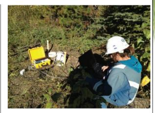
collar, while the automated long-term multiplexing system can be deployed for months, with up to 16 chambers in an area of 30 meters in diameter. In addition to  $CO_2$ , other gases can be measured with the LI-8100A System by adding an auxiliary gas analyser or taking air samples from the chamber head space for analysis back at the laboratory.
