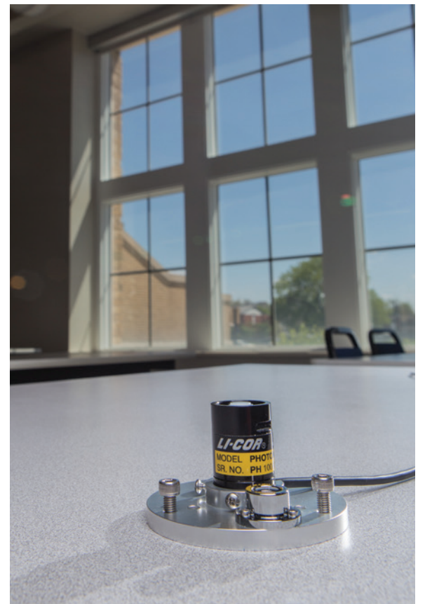
Figure 3: Photometric sensors are sensitive to light as perceived by the human eye and are used to optimise lighting.
