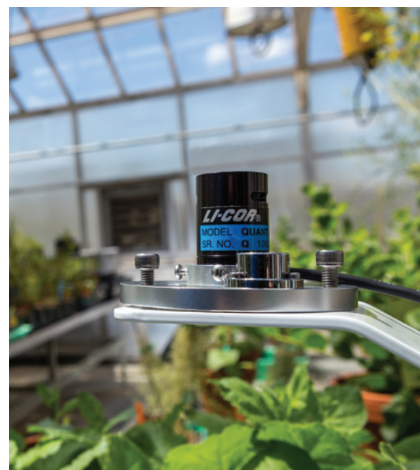
Figure 2: Quantum sensors can help optimise lighting conditions in greenhouse applications.
