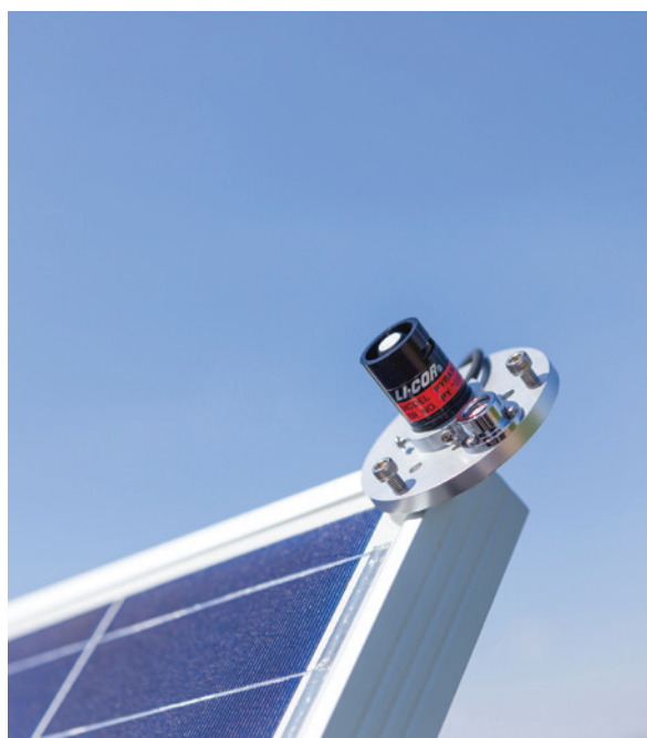
Figure 1: Pyranometers are used to assess solar energy potential and efficiency.
