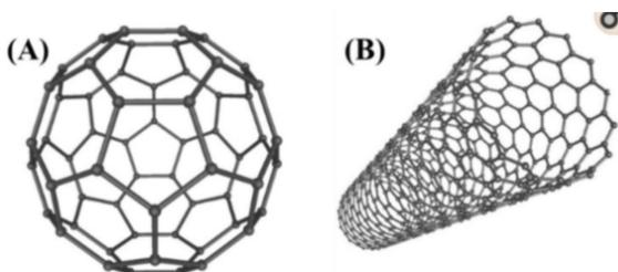
Figure 1: (A): C60 (fullerene), (B): carbon nanotubes
