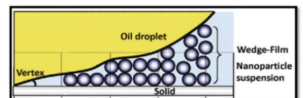
Figure 3: Nanoparticle structuring in the wedge-film [10]
