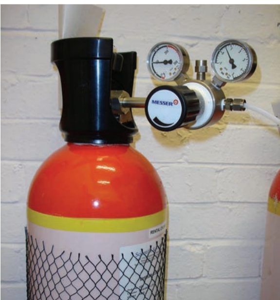
Figure 4: Typical delivery systems for calibration gas
