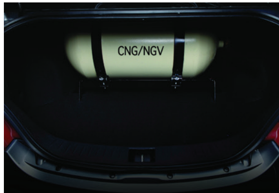
Automotive CNG tank in car boot
