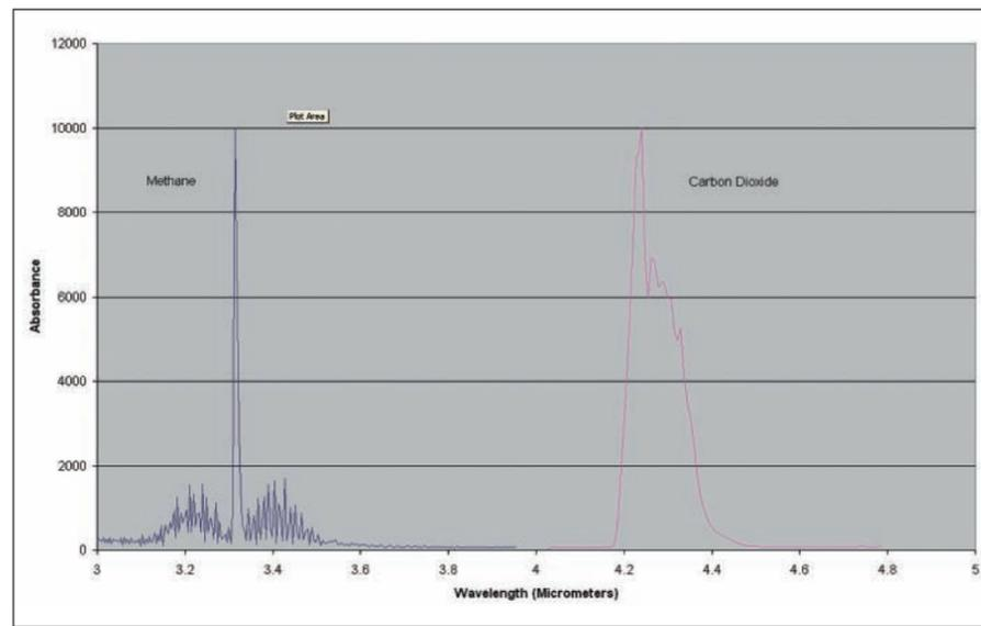
Figure 3, Absorption bands of Carbon Dioxide and Methane
