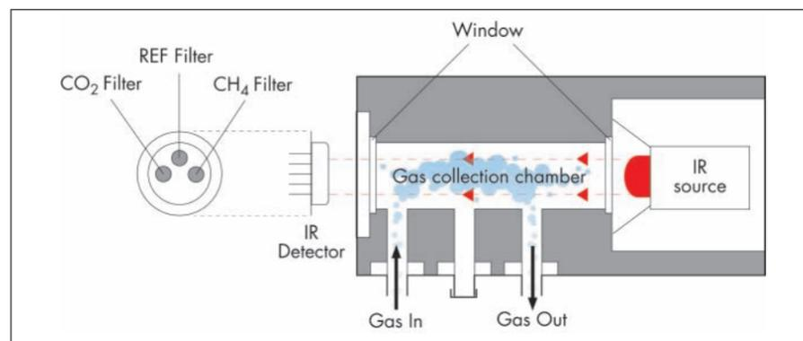
Figure 4, Infrared cell
