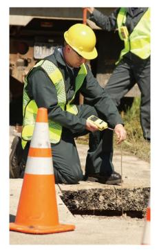
However, it is not enough to take your gas monitor, make a quick check of the atmosphere, and throw your instrument back under the seat of the truck. Atmospheres in construction environments can change quickly and danger can come at any time. The only way to guarantee full time protection on the job, is to have the instrument working for you for the entire job.
