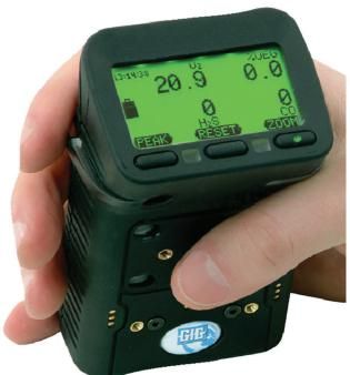
Figure 1: Always allow all of the sensors installed in your instrument to stabilise completely in fresh air BEFORE making a fresh air zero adjustment.
