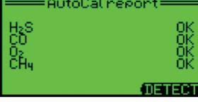
Figure 4: GfG instruments can be automatically fresh air zeroed or calibrated by means of a simple "AutoCal®" procedure, (press "Air" to make an automatic fresh air zero adjustment, "Gas" to make a span calibration adjustment, or "Exit" to return to normal operation)
