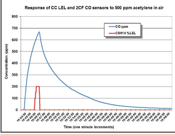
Figure 3: Electrochemical CO sensors can take a long time to clear after exposure to certain interfering contaminants such as acetylene.
