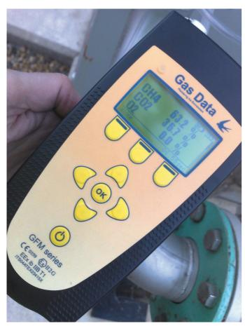
The GFM435 sets a high standard. Having a comprehensive MCERTScertification it really is the ultimate landfill/remedial site meter. The analyser measures gas concentrations, but it also measures pressures, flows and temperatures and because of this it can be used to equally great effect at peripheral boreholes and gas extraction wells.
