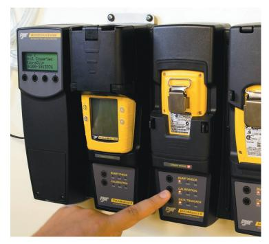
The automatic generation of paper work such as fleet status reports and calibration certificates can also be greatly reduced with devices like MicroDockII when combined with Fleet Manager II software; data can be downloaded with a single button press and a few minutes wait using the device's data logging facility and this information can be easily converted into a variety of reports by using the intuitive software interface and a PC.
