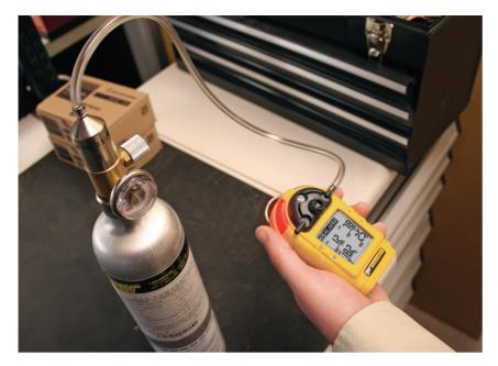
are absorbed by the active sensor catalyst and the sensor response can be inhibited. Sensor inhibitors create a loss in sensitivity to combustible gases, however, exposure to these compounds is typically temporary and once the detector is removed from the contaminated environment the sensor will recover normal sensitivity. In some cases, chronic exposure to inhibitors will permanently damage the catalytic bead combustible sensor.
