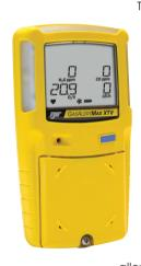
Testing the atmosphere of a confined space at all levels is essential as some gases are heavier than air (such as  $H_2S$ , which is slightly denser than air), some lighter (such as  $CH_4$ ), and some the same density (such as CO). It's important to use a multi-gas detector capable of monitoring for the gas hazards expected to be in the location in question.
