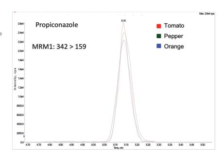
Figure 5: Propiconazole at 10  $\mu$ g·kg<sup>-1</sup>, diluted 30 times, in three different matrices analyzed by a 4500 AB SCIEX QTRAP LC-MSIMS system. The HPLC system used was the Eksigent ekspert™ microLC 200, equipped with a Halo C18 column, 0.5 x 50 mm, and a 2.7µm particle size at 30 °C (Eksigent, AB SCIEX Instruments, Foster City, CA)
