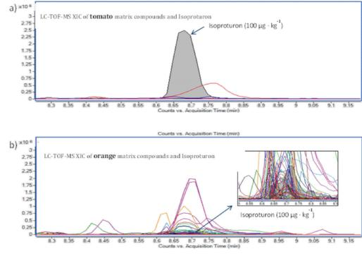
Figure 4: Extracted ion chromatogram of Isoproturon (m/z 207.1492) and co-eluting matrix compounds in tomato (a) and orange (b). Analyzed by a 6530 Agilent LC-QTOF-MS. The HPLC system used was the 1200 series from Agilent Technologies, equipped with a XDB-C18 analytical column of 4.6 mm × 50 mm and a 1.8 µm particle size
