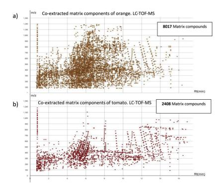
Figure 3: Matrix compounds of orange (a) and tomato (b) extracts analyzed using a 6530 Agilent LC-QTOF-MS. The HPLC system used was the 1200 series from Agilent Technologies, equipped with a XDB-C18 analytical column of 4.6 mm × 50 mm and 1.8 µm particle size
