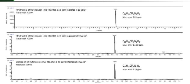
Figure 7: Detection of pesticide flufenoxuron at 10  $\mu$ g·kg<sup>-1</sup>in tomato, pepper and orange. Resolution 70000, mass tolerance of 5 ppm. Analyzed by Orbitrap QExactive (ThermoFisher Scientific, Bremen, Germany) mass spectrometer. The UHPLC system used for these tests was the Dionex Ultimate 3000. It was equipped with an Thermo Accucore C18 column 150×2.1mm; 2.6  $\mu$ m particle size held at 25 °C
