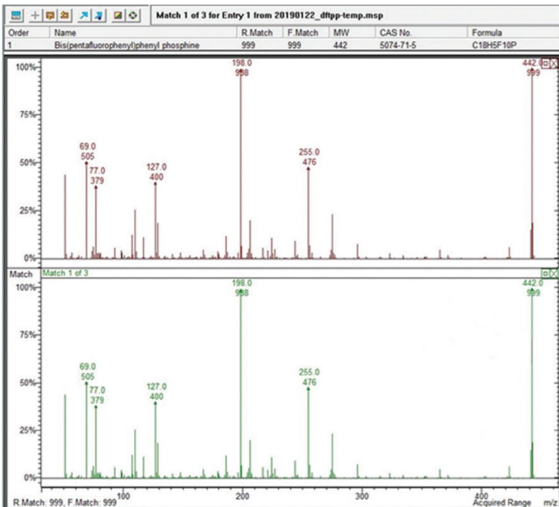
Figure 2. Mass spectra of DFTPP tune sample against NIST library
