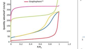
Figure 1. N2 Adsorption isotherms for Supelco® carbons.
