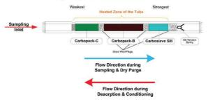
Figure 7. Multi-bed tube for air sampling (Carbotrap® 300).
