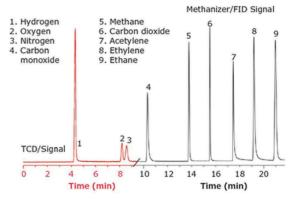
Figure 4. Separation of permanent gases and light hydrocarbons with a Carboxen® 1010 PLOT column.
