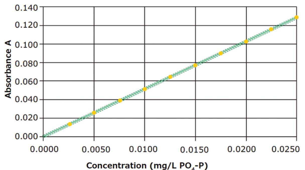
Figure 2: Calibration curve for the measurement range 0.0025 – 0.0250 mg/L PO<sub>4</sub>-P
