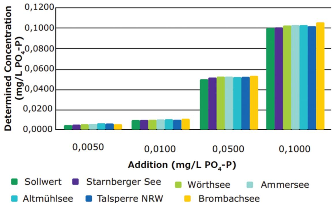
Figure 1: Orthophosphate concentration recovered after standard addition
