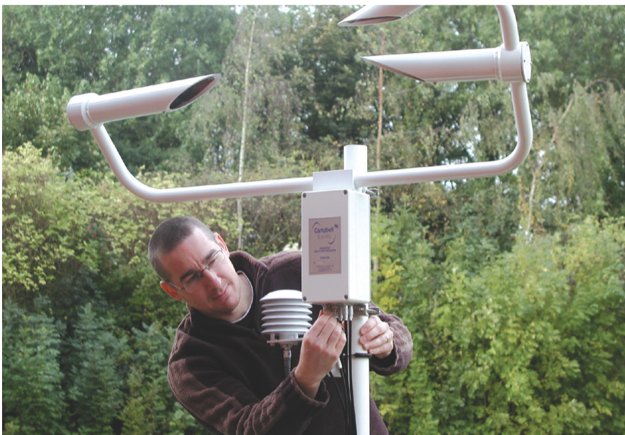
Figure 1. The Campbell Scientific PWS100 being installed.
