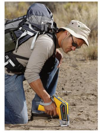
Portable XRF analysers are employed in remediation work to guide earth-moving equipment to soil contamination 'hotspots' which results in less soil removal and thereby lowers costs. These instruments can perform both in-situ (on site) and ex-situ soil analysis (analysing prepared soil samples, via the prepared sample test-stand and soil sample preparation kit). This reduces the costs and time incurred by laboratory analysis.
