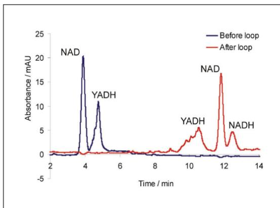
Figure 4. Electropherograms obtained in the single run, before and after the reaction loop, showing conversion of NAD to NADH in the process catalyzed by yeast alcohol dehydrogenase (YADH).
