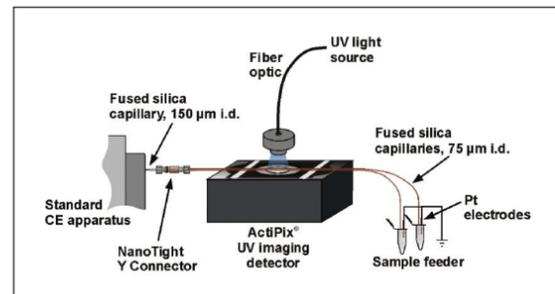
Figure 2a. Parallel capillary electrophoresis: coupling of two capillaries to a commercial CE system using a low volume Y-connector (Upchurch)
