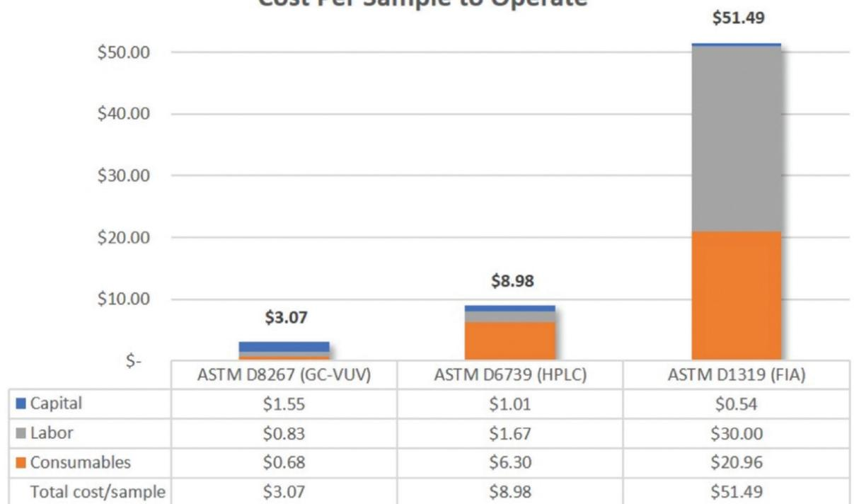
Figure 3: Cost per sample comparison for GC-VUV with HPLC and SFC.
