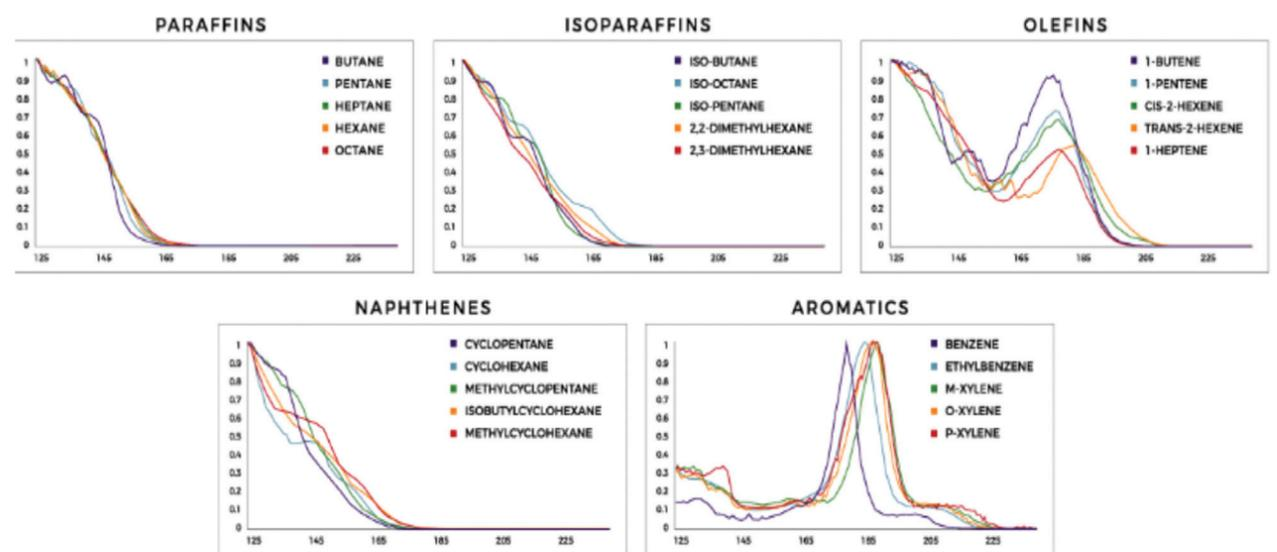
Figure 2: Example VUV Spectra showing unique compound specific and hydrocarbon class similarities for a selection of common molecules encountered in fuels
