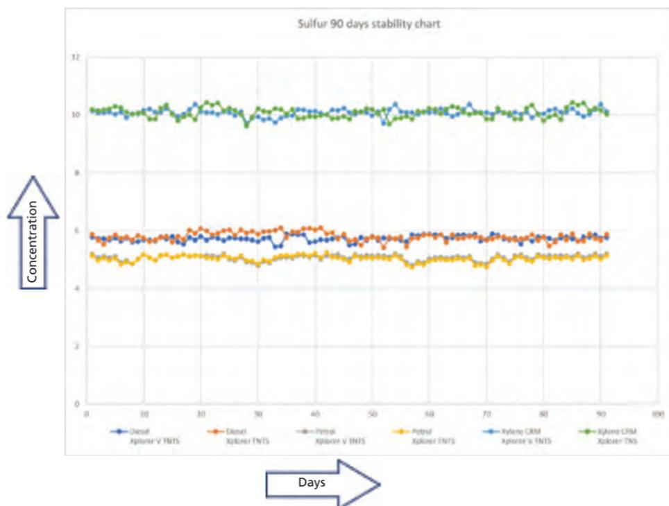
Sulfur: Calculated final Tier 3 results for precision and accuracy on Sulfur, 90 day run
