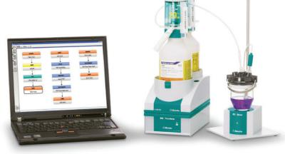
Figure 1. The 859 Titrotherm with magnetic stirrer, two Dosinos, and the tiamo™ software: This simple setup allows you to measure the acid number of crudes and refinery fractions.
