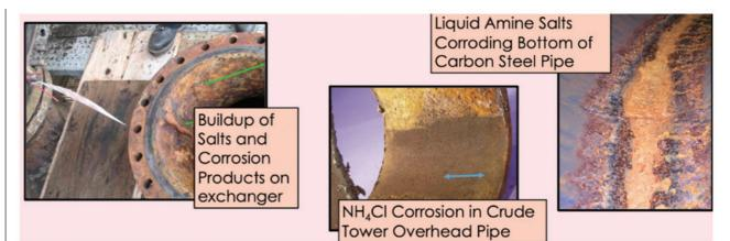
Figure 1: Excessive chloride left in the crude resulting in corrosion of equipment [11]
