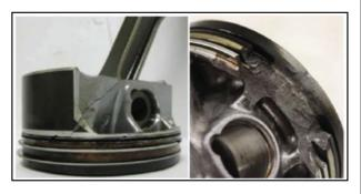
Two examples of piston damage due to LSPI
