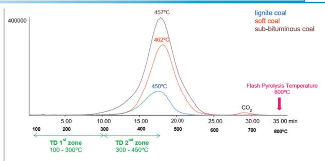
Figure 3. Overlaid EGA Thermograms with Peak Top Temperature (Shiono et al. 2013)
