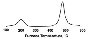
Figure 2. Example of an EGA Thermogram ("Evolved Gas Analysis (EGA)," 2019)
