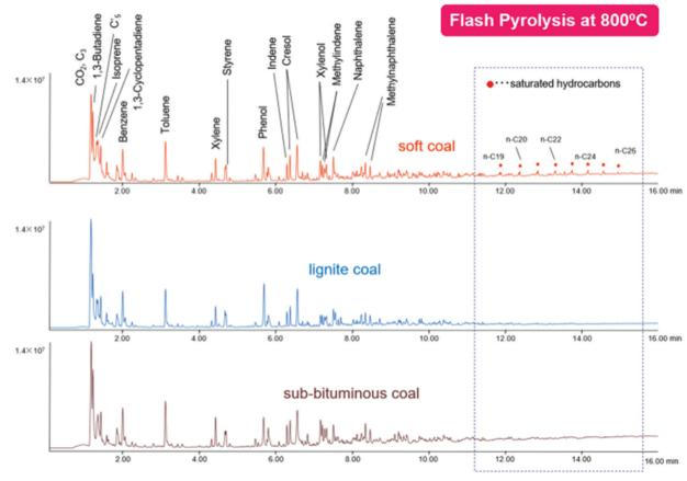
Figure 4. Flash Pyrolysis Pyrograms of Coal Samples (Shiono et al. 2013)
