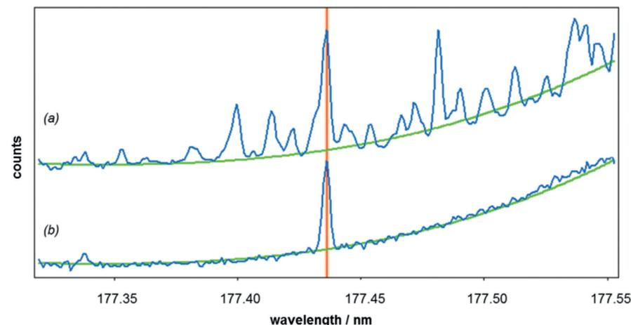
Figure 3: High resolution optical emission spectra of P 177.436 nm (orange line) recorded on PlasmaQuant® PQ 9000 in an oil-xylenes mixture (a) without and (b) with correction of spectral interferences (CSI). Green lines represent the automatic baseline fitting (ABC).
