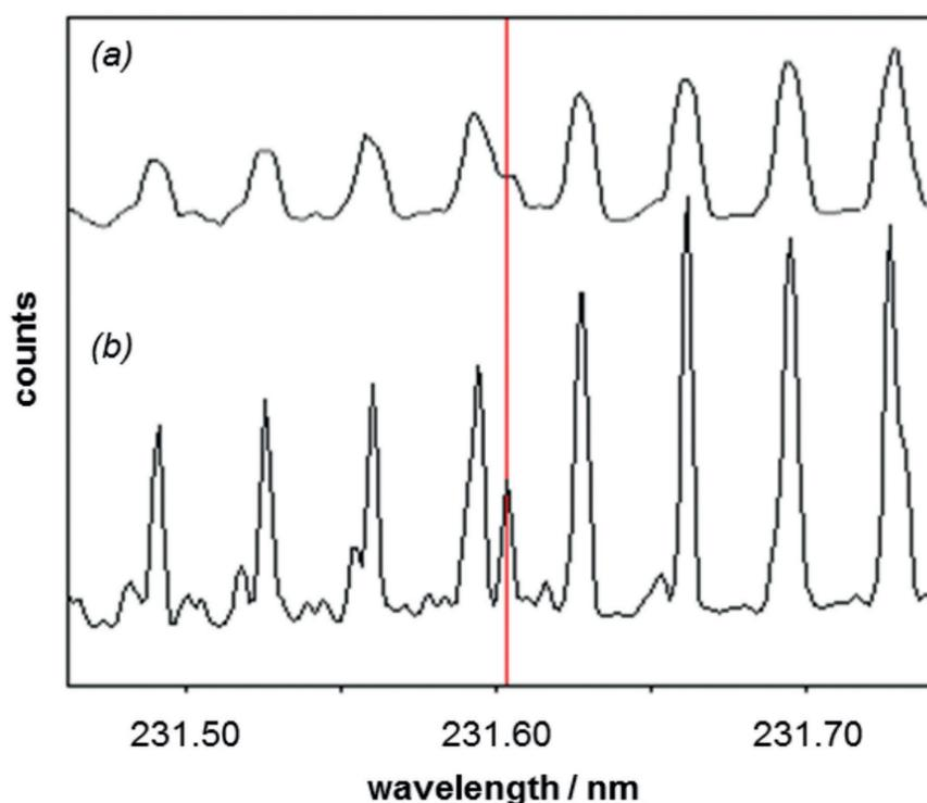
Figure 2: Comparison of Ni 231.603 nm (1 ppm, red line) in an oil-kerosene mixture recorded on ICP-OES instruments with (a) conventional and (b) high spectral resolution
