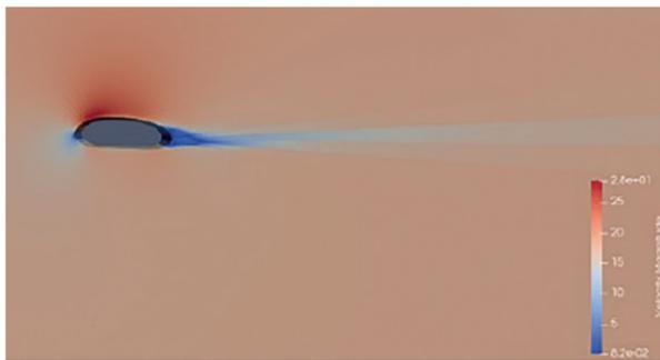
Figure 2. Screenshot of a sample CFD result, showing the surrounding velocity magnitude for a cruise speed of 18 m/s around the UAV body.
