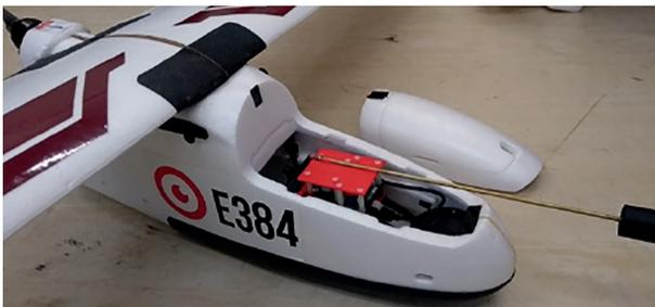
Figure 4. E384 payload bay with instrument.
