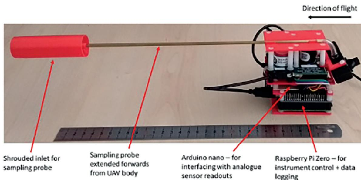
Figure 3. Assembled instrument with a prototype inlet for isokinetic sampling in flight
