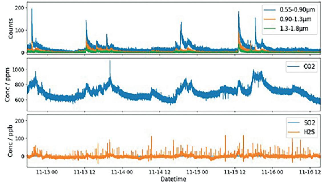
Figure 5. Test results from running the instrument in a domestic environment.
