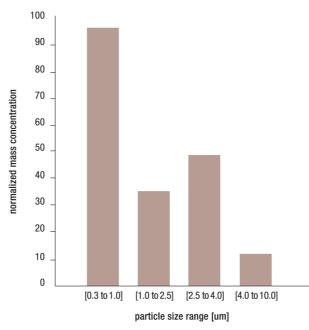
Figure 4: Particle composition of smoke (Source: Sensirion)
