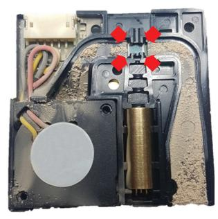
Figure 6: Clean photodiode after stress test (Source: Sensirion)
