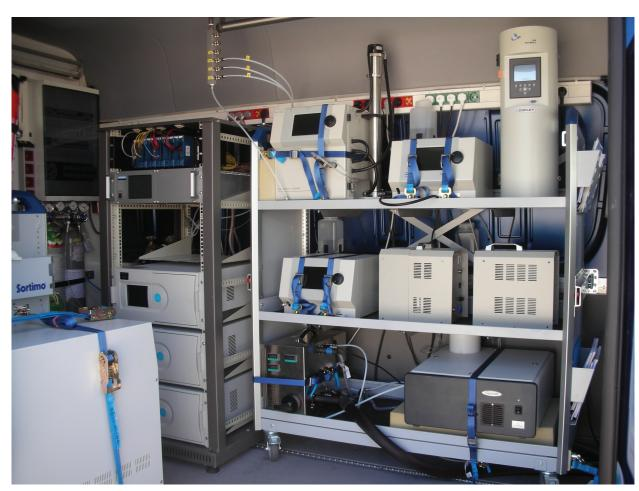
The van interior is fitted with analysers for both engine emissions monitoring and ambient air quality
