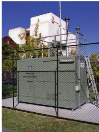
These monitoring stations measure “criteria” pollutants, which are gases that include O<sub>3</sub>, CO, NO<sub>2</sub>, SO<sub>2</sub> and particulates such as PM10 and in some countries PM2.5.
